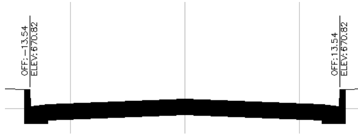
Figure 9. This example shows Top_Curb codes being used to label cross sections. Offsets and elevations are automatically derived from the corridor model and conform to company or jurisdictional CAD standards.
